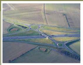
Baldersby East and West Ponds visible highlighting forebay with reeds and secondary dry retention storage area, Junction 50 A1(M)
