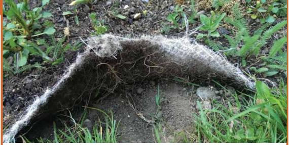
Vegetation mat starting to disintegrate, and poor vegetation establishment
