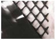
Geocomposite forms a drainage layer
