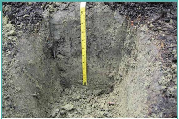
Figure 21.3 Anaerobic soil conditions within layer of topsoil
