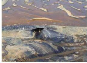
Poorly-welded joint, with geomembrane gathering creating gap in seal
