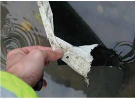
Tape from DIY store used to seal geomembrane instead of welding, leading to leaks
