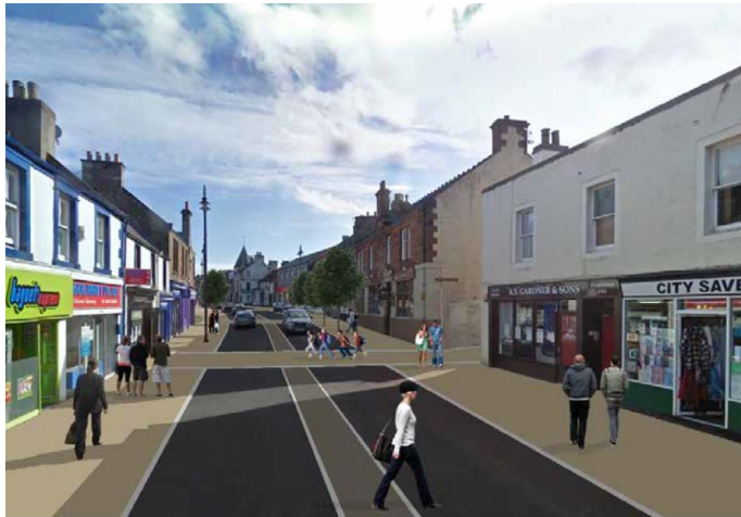
Indicative sketch from charrette report on how Tranent High Street might look without parked vehicles and with wider footways. Priority is given to the pedestrian with vehicle movement slowed by narrow lanes and crossing points.
