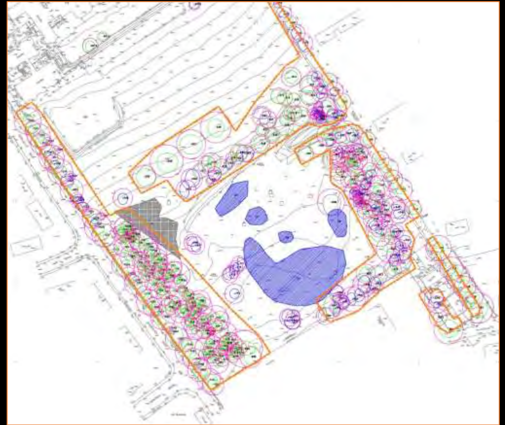
Tree Survey - Tree Root Protection Zone
