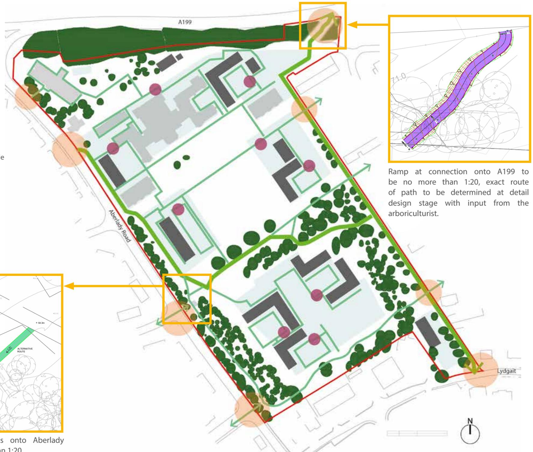
Ramp at connection onto A199 to be no more than 1:20, exact route of path to be determined at detail design stage with input from the arboriculturist.
