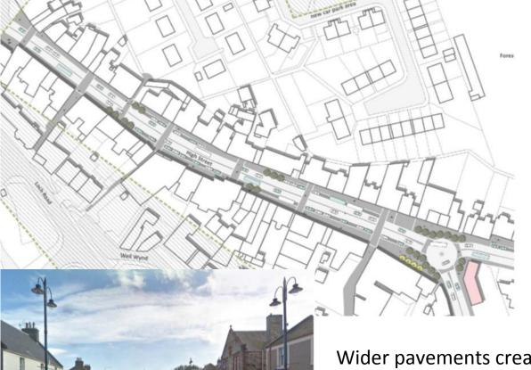
This begins with vehicle attenuation zones at either end of High Street that physically signal to drivers that they are entering an area with a different set of 'rules'. Vehicle lanes are narrowed through widening the pavements and introducing a median strip, again to slow down drivers.
