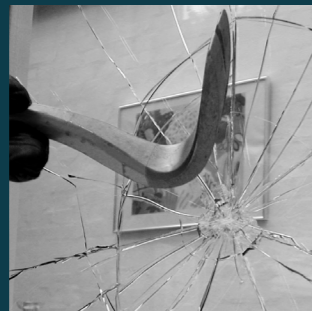
The length of time it takes to break a laminated pane will discourage even the most persistent burglar.
