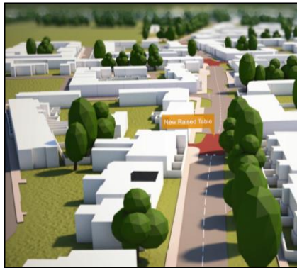
Figure 1 – New Street to become a quiet street with raised tables (a raised section of road that's ramped on each side to make crossing easier) at junctions. All parking would be kept
