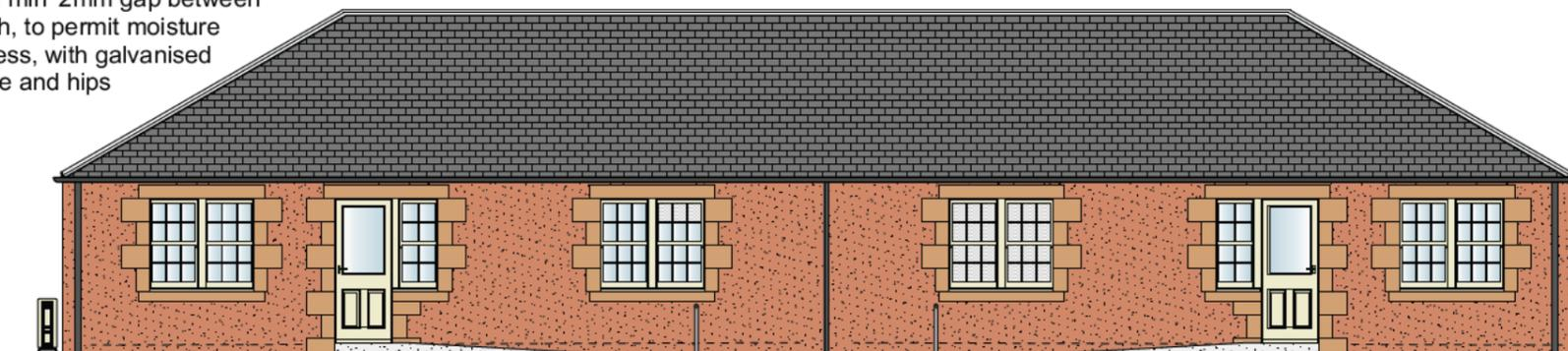
traditional roughcast walls (colour to be agree with ELC) with Corshill stone or equivalent rybats, sills & lintels around openings
