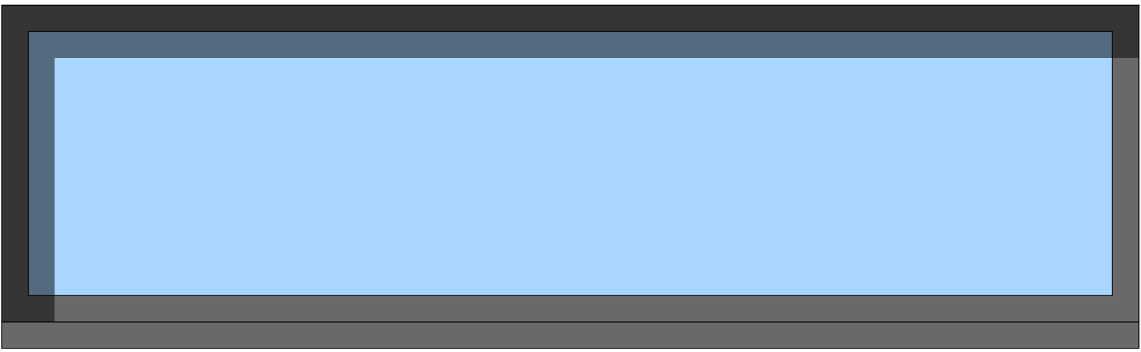
Rear elevation (North) GFL window Grey aluminium Clear double glazed Fixed
